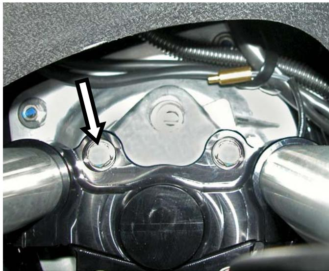
Loosen bolts securing upper to riser tubes (2 per side).
