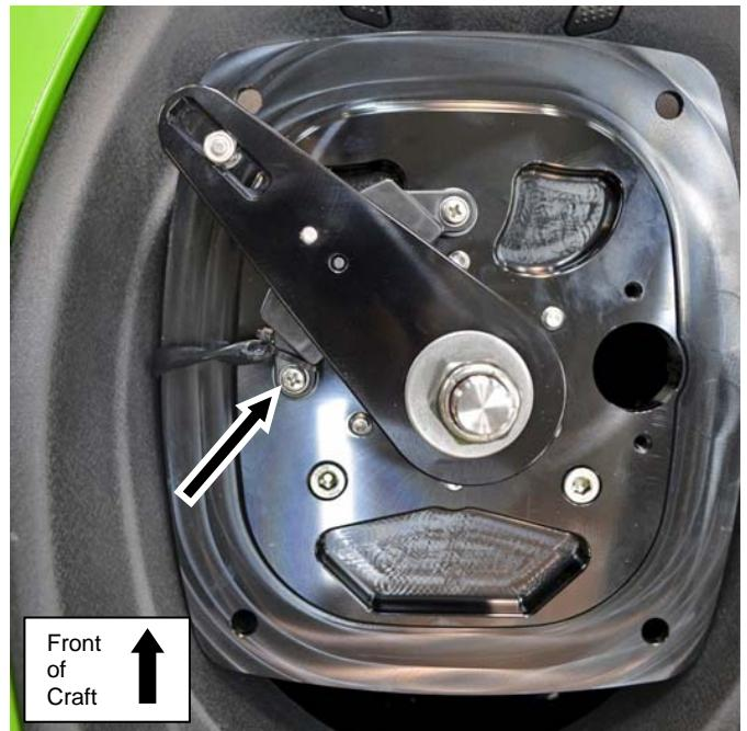
Mount Steering System Lower onto hull and secure using stock hardware (4 nuts & washers). **NOTE: Apply red Loctite to threads. Do not over tighten nuts.**
