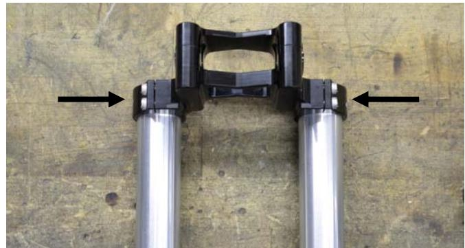
Carefully slide upper down on riser tubes.
