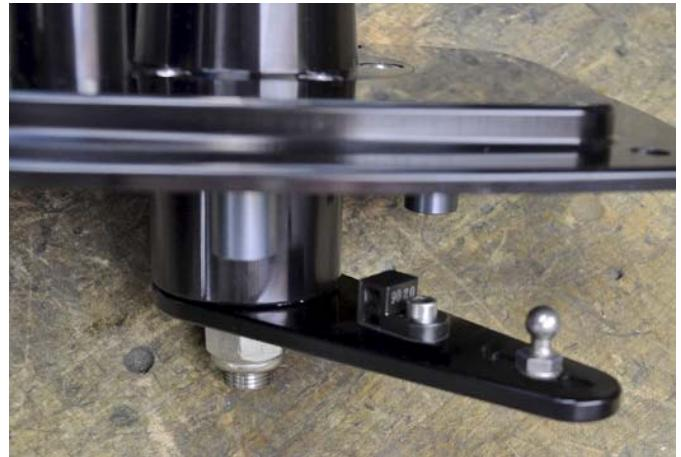
**TIP:** For faster steering move ball joint in towards steering shaft. For slower steering move ball joint out towards end of steering arm. Center for stock steering setting.
