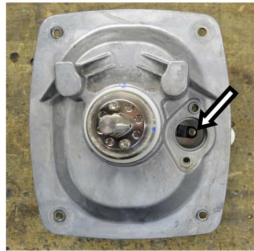
Remove Off Throttle Steering magnet (1 screw).
