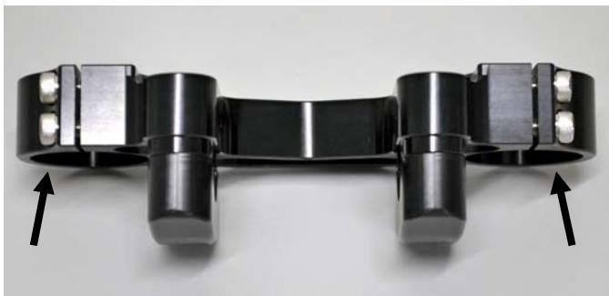
Carefully slide one riser tube up into lower until flange or riser tube stops against lower. Remove bolts, apply red Loctite and secure. **NOTE: Do not over tighten bolts.**
